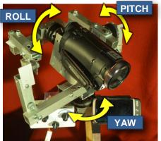
As a remote control for the gimbal, I built a second control box with a 5 m long cable which replaces the above mentioned controls automatically when the cable is connected. Also this remote control box has a mobile phone holder. So I can place the gimbal somewhere in my boat up to 5 m away from the place where I am sitting, and I can control the gimbal as well as the camera while the camera records pictures of me.
